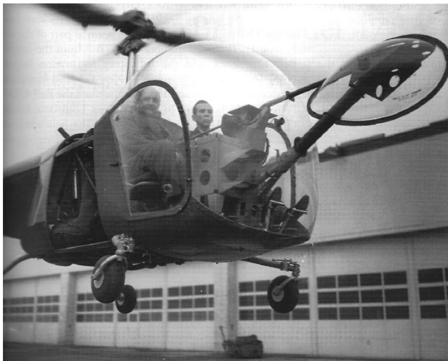
Bell 47B2 helicopter showing the magnetometer attached to the front of the bubble. Bell pilot Jay Demming is in the left seat (on the right in the photo) and Hans Lundberg is seated next to him (source: Bell Helicopter/ Jeff Evans and Ned Gilliland Collections).
